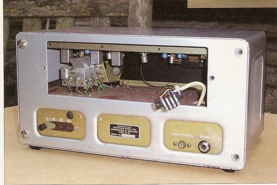
The back of the EC10 showing the space for the mains power supply unit.
